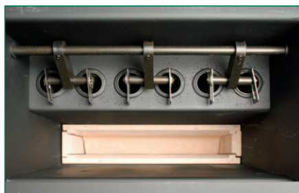
Heat exchanger with cleaning
